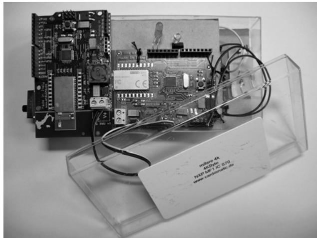
**Figure 1. Prototype of an Audio-tactile Location Marker developed as auxiliary enhancement of tags.**
