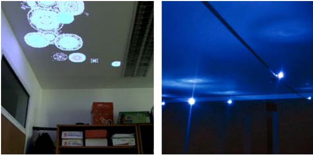
Figure 3. The peripheral weather application showing cold temperature and rainfall (left) and the sound-responsive ceiling display visually reflecting the sound level inside a space (right)
