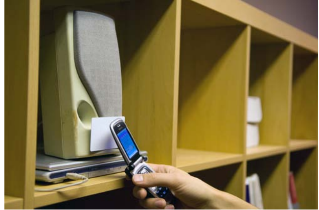
Figure 2. The ALM prototype used for the evaluations, which consisted of a laptop, a speaker, and an NFC tag. The picture also shows the mobile phone interaction with the prototype.
